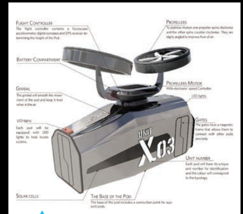
Each pod will utilize advance propeller technology similar to drones, and gyroscopic controls to create a viable functional clinical environment.
