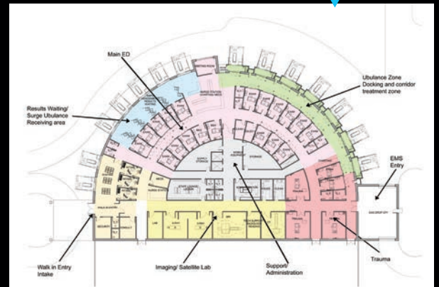
Prototype ED showing docking area for "ubulance" and additional surge receiving areas.
